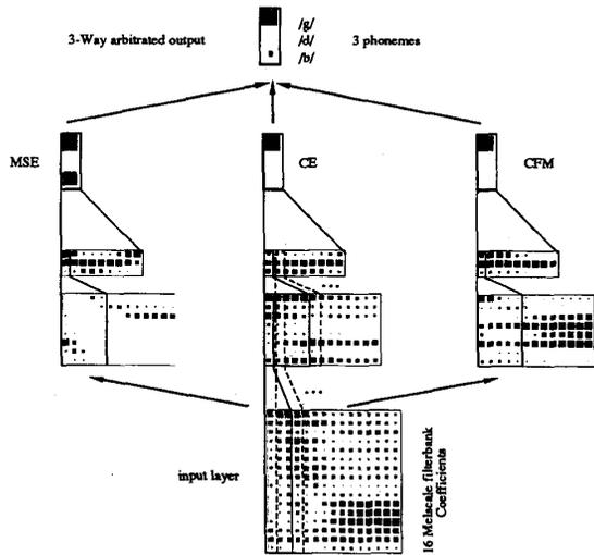
Fig. 11. Three-way conflict arbitration using TDNN's trained with the MSE, CE, and CFM objective functions. Note that the ambiguous MSE output is corrected by the arbitration scheme.
