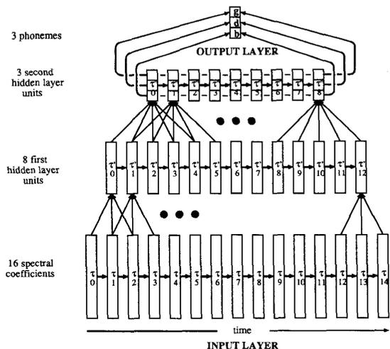
Fig. 1. A time-delay neural network (TDNN) block diagram.
