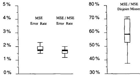
Fig. 13. A graphic summary of an MSE/MSE conflict arbitration control experiment on speaker MAU: error rates and percent disjoint misses (MSE:  $n = 6$ ; MSE/MSE:  $n = 15$ ).
