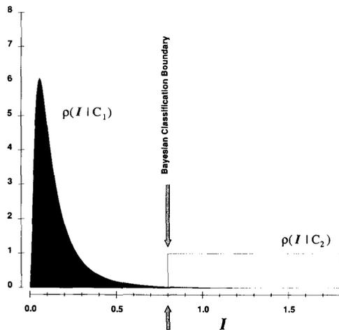
Fig. 14. Class conditional densities for a two-class problem (with equal class "priors").
