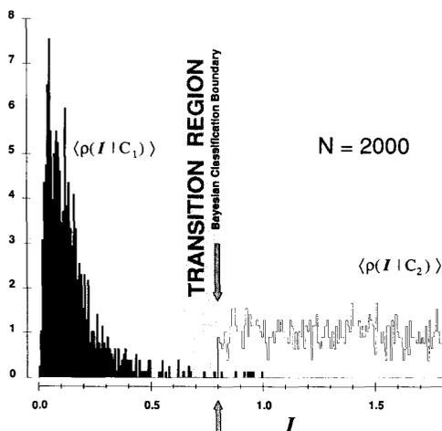
Fig. 15. A sample training set for the two-class problem; 1000 samples are drawn from each class.
