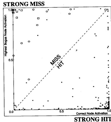
Fig. 10. Scatter plot of arbitrated MSE/CFM classifier outcomes.  $\square$  indicates post-arbitration miss correctly classified by MSE.  $\circ$  indicates post-arbitration miss correctly classified by CFM.
