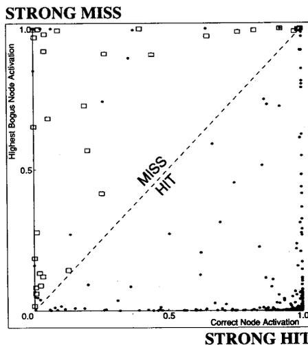
Fig. 8. Scatter plot of CFM classifier outcomes.  $\square$  indicates CFM miss correctly classified by MSE.
