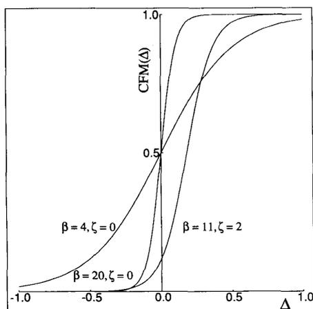
Fig. 4. CFM plotted for representative parameter values:  $\alpha = 1.0$ ,  $\beta = 4.0$ ,  $\zeta = 0.0$ .
