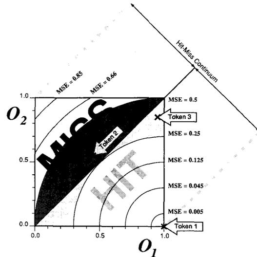
Fig. 3. A contour plot of MSE for a two-output network; output  $\Theta_1$  represents the correct class.
