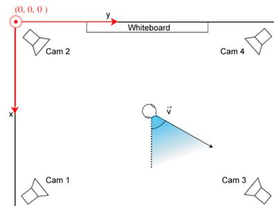
**Figure 2. Four cameras are placed at the corners of the smart-room, such that at least one facial view of the head can be obtained. We estimate the horizontal rotation angle (pan) of a person's head by combining the estimates from multiple cameras.**
