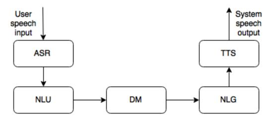
Figure 2.1.: A typical architecture pattern for a SDS
