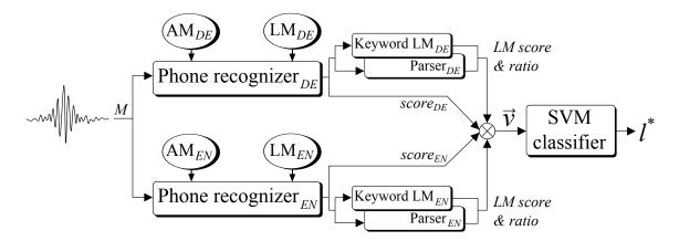
Figure 5.1: Schematic of our enhanced PPR system. Additional language cues are scores of the generic language-dependent keyword n-gram models and a keyword phones to hypothesis length ratio.
