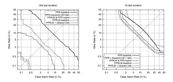
Figure 5.4: DET curves illustrating the performances of the PPR and PPRLM baseline systems and hybrid system, as well as the performance improvements of the modified systems. The PPRLM systems and PPRLM & PPR hybrid use language model scores. Depicted are the observations on the 30s test segments (left) and 3s test segments (right).
