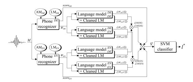
Figure 5.3: Schematic of our proposed hybrid system, utilizing the phone recognizer frontends of the PPR approach, and the language model scoring back-ends of the PPRLM framework. The language cure vector  $\boldsymbol{v}$  is generated by stacking both, the phone recognizer scores and combined and averaged language model scores.
