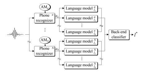
Figure 3.3: Schematic of a parallel phone recognition followed by language modeling (PPRLM) system, using several PRLM subsystems in parallel. Classification is done via averaged language model scores, combined in a language-wise fashion [AD10].
