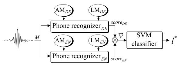
Figure 4.1: Schematic of our PPR system, using German and English phone recognizers. Classification is done by an SVM back-end classifier and the Janus-specific recognizer scores, stacked to a language cue vector  $\vec{v}$ .
