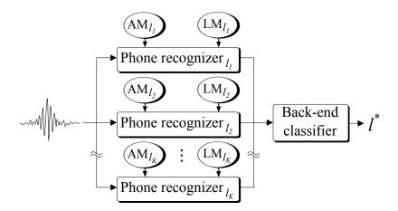
Figure 3.1: Schematic of a parallel phone recognition (PPR) system, which incorporates language models for language-dependent phone-based decoding and uses the recognizer scores for classification [AD10].
