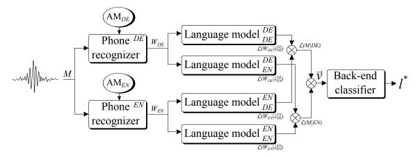
Figure 4.2: Schematic of our PPRLM system, using German and English phone tokenizers. Classification is done by an SVM back-end classifier and the combined and averaged language model sentence scores, stacked to a language cue vector  $\vec{v}$ .
