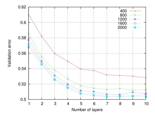
Figure 5.3: Dependence between the number of layers and validation error
