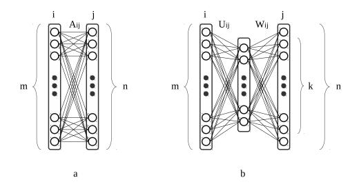
Figure 4.1: An example of SVD applied to a weight matrix in a DNN. **a**: matrix before SVD. **b**: matrix after SVD
