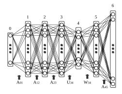
Figure 4.5: An insertion of bottle-neck layer to DNN with 4 hidden layers
