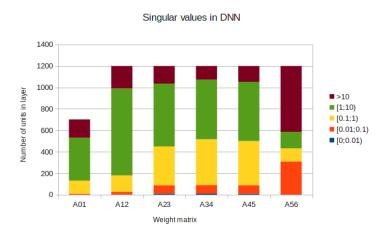
Figure 5.5: Analysis of singular values of DNN with 5 hidden layers
