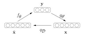
Figure 2.4: An example x is corrupted to  $\tilde{x}$ . The autoencoder then maps it to y and attempts to reconstruct x[VLBM08].
