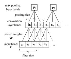
Figure 2.6: Diagram showing a typical convolutional network architecture consisting of a convolutional and max-pooling layer. In this diagram, weights with the same line style are shared across all convolutional layer bands [SMKR13]
