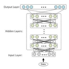
Figure 2.9: DNN used in ASR systems [XLG13]
