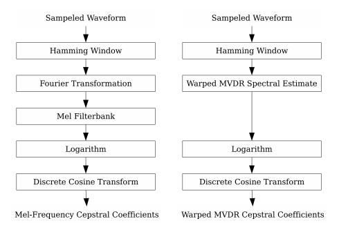
Figure 2.2: Block diagrams illustrating all the processing steps required for the calculation of the compared mel-frequency cepstral coefficient and warped MVDR cepstral coefficients front-ends [VSR12]
