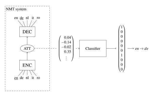
Figure 4.1.: Schematic description of the procedure we use to test for the dependency of the context vectors. During translation the context vectors are extracted from the attention module, and fed to the classifier. The classifier output is a "two-hot" vector representing the predicted source and target language in the its first and second half (every language is assigned a fixed dimension, e.g. English in dimension 0,...).
