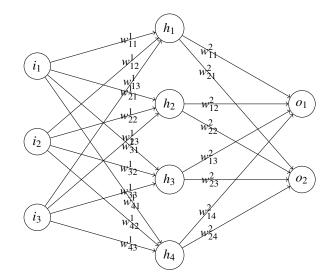
Figure 2.1.: A Simple Feed Forward Network with one hidden layer, 3-dimensional input, 2-dimensional output and fully connected layers
