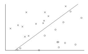
Figure 2.3.: Example of a linearly separable set of data points with two classes represented by circles and crosses
