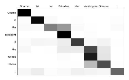
Figure 2.8.: Exemplary word alignment represented as alignment matrix (generated by one of the NMT systems trained for our experiments)
