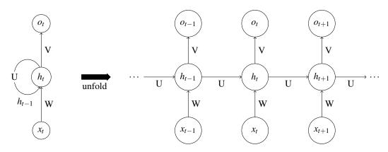
Figure 2.5.: In backpropagation through time in order to apply backpropagation to an RNN, the RNN is unfolded after having been applied to an input sequence. As a result the originally unique weights are found present multiple times.
