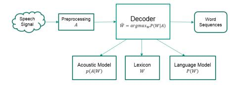
Figure 2.1: Components of a typical ASR system, the input of an ASR system is the speech signal and the output is the best matched word sequence.
