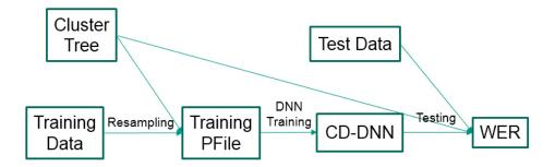
Figure 5.3: The test setup for the cluster trees. With cluster trees the polyphone states in the alignments of training data are replaced with the leaves in cluster trees (senones). A CD-DNN can then be trained based on these alignments. The trained CD-DNN is integrated into an ASR system as the acoustic model, the final ASR system is tested on test data, and the results can be represented by WERs. Generally by comparing WERs, we compare the performance of different acoustic models.
