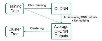
Figure 5.1: The pipeline to build a DNN based cluster trees. The start point is training data accompanied by frame-to-state alignments. A CI-DNN can be trained based on these alignments, after that we can calculate the average CI-DNN outputs for each quinphone state using the CI-DNN. Finally the clustering algorithm can be performed based on the average CI-DNN outputs, and the end result is the phonetic cluster trees.
