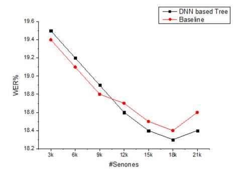
Figure 6.1: Test results of implemented ASR systems. Both the DNN based approach and the GMM based approach achieved lowest WERs with 18k senones; the DNN based tree with 18k leaves had a WER 18.3% which was lower than the WER of the GMM based tree.
