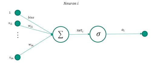
Figure 3.1: Structure of an artificial neuron, the bias of a neuron can also be regarded as the weight of an input with a constant value of one.
