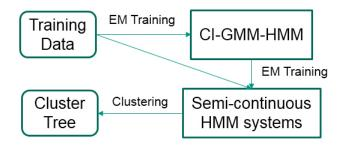
Figure 5.2: The pipeline for building a conventional GMM based cluster tree. The first step is to train a CI-GMM-HMM system, and then the context independent system is extended to a context dependent semi-continuous HMM system, finally the mixture weights of the semi-continuous HMMs are used to build the cluster trees.
