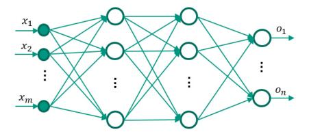
Figure 3.2: Architecture of an MLP with m input neurons, two hidden layers and n output neurons.
