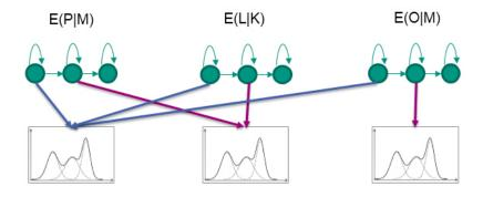
Figure 2.5: State tying: different HMM states can be tied to the same GMM.
