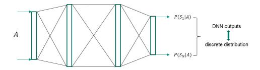
Figure 4.1: The architecture of a CI-DNN with two hidden layers, where  $S_1, ..., S_N$  are monophone states. The input of a CI-DNN is the feature vector A, the output is the a posteriori probabilities of HMM states.
