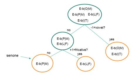
Figure 2.6: An example of the cluster tree for the triphone states derived from the monophone state E-b.
