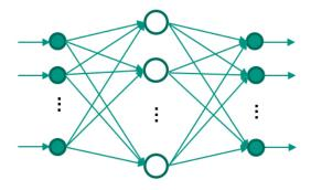
Figure 3.3: Architecture of an autoencoder, the input and output layers have the same size.
