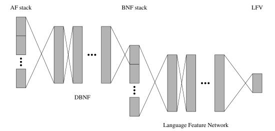
Figure 1: Overview of the network architecture used to extract language feature vectors (LFV). The acoustic features (AF) are being pre-processed in a DBNF in order to extract BNFs. These BNFs are being stacked and fed into the second network to extract LFVs.
