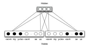
Figure 3: A bigram letter index RBMLM with three hidden units and two word contexts, where activated units are marked as black.
