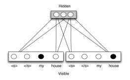
Figure 2: RBMLM with three hidden units and a vocabulary size of two words and two word contexts, where activated units are marked as black.
