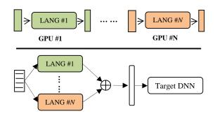
Figure 2. DistLang for distributed feature extractor learning. Top: each GPU trains a feature extractor on each language. Bottom: on the target language, outputs from individual extractors are fused into a unified feature representation.
