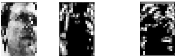
Figure 3: Preprocessed images: normalized grayscale, horizontal edge and vertical edge image (from left to right)
