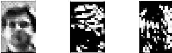
Figure 5: Preprocessed images: normalized grayscale image, horizontal and vertical edge image (from left to right)
