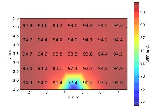
Figure B.1.: Word error rate depending on the receiver position in the classroom for the baseline system. The system cannot deal with reverberation except when directly in front of the speaker. Even then it is falls short to the system trained with one or more RIRs from the classroom.
