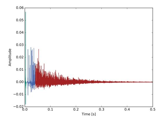
Figure 2.13.: Example of a measured room impulse response (RIR) with the direct soundpath (green), early reflections (blue) and late reflections (red) and  $T_{60} = 0.7$ . The impulse of direct-path sound is not always clearly visible.
