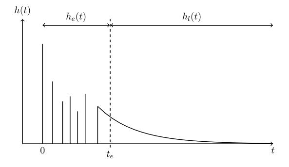
Figure 2.12.: Schematic view of a RIR. The impulse response h(t) is split into two parts  $h_e(t) h_l(t)$  by the boundary  $t_e$ .
