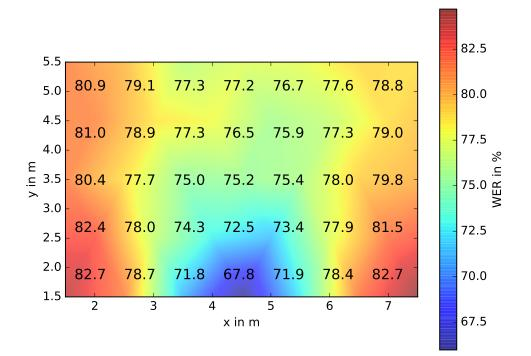
Figure B.2.: Word error rate depending on the receiver position in the classroom for a system trained with a single RIR from the middle of the room.
