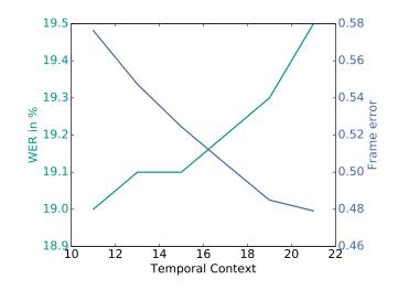
Figure 5.2.: WER (blue) on tst2013 and frame classification error (green) for DNN acoustic models with different temporal context. The context is given as number of frames and is always symmetric (e.g. context 13 indicates that the network it given the features from frame t - 6 to t + 6). The system was trained with clean speech.
