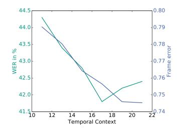
Figure 5.3.: WER (blue) on tst2013\_rvb and frame classification error (green) for DNN acoustic models with different temporal context. The models were trained on reverberated audio from measured RIRs.
