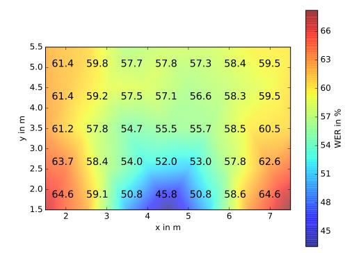
Figure 5.1.: Word error rate depending on the receiver position in the classroom. The acoustic model was trained with 100 RIRs from the room and tested on the remaining 30 RIRs. The background color is a linear interpolation between the measurement points. It is not said that the WER degrades linearly, but the visualization highlights that the WER does depend on the distance and the microphone angle. The speaker is positioned at x = 4.5 and y = 0.5.
