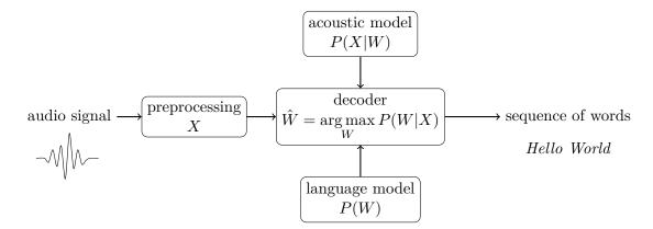
Figure 2.1.: Flowchart of a speech recognition system
