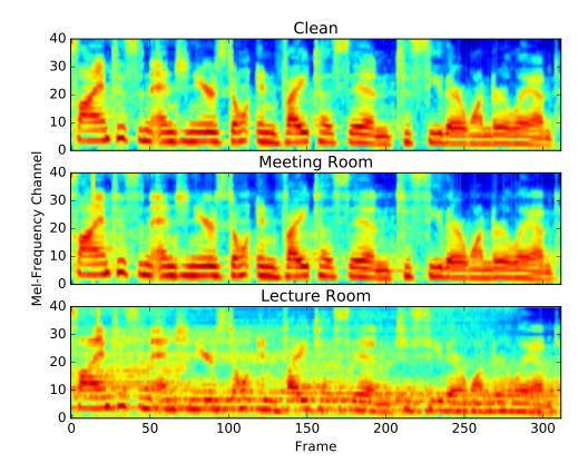
Figure 1.1.: Mel frequency spectrum for the same sentence spoken into a close-talk microphone and two distant microphones a few meters into big rooms. The spectrum and especially the formats get smeared in time.
