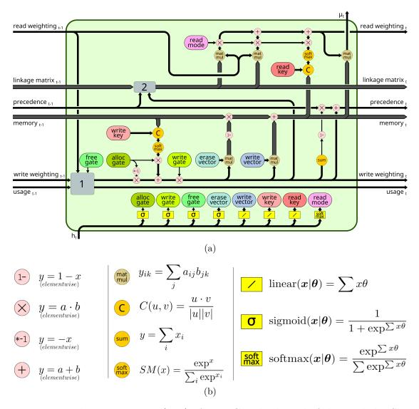
Figure 2.15: The memory unit (MU) of a DNC and a legend of the symbols. Slim arrow lines are scalar transitions, medium lines are vector transitions and wide lines are matrix transitions. The gray blocks are summarized functions. Horizontal outgoing lines are recurrent connections within the MU.
