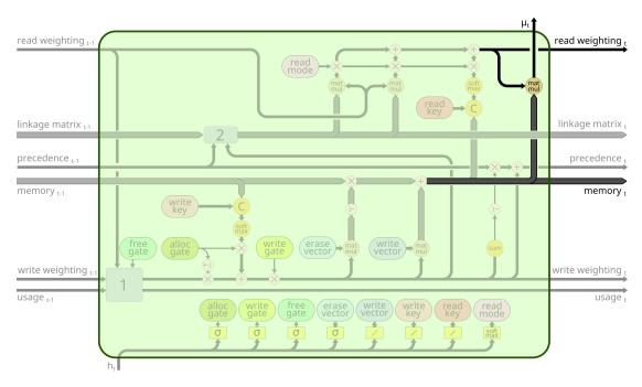
Figure 2.22: The illustration of the memory reading of one read head.
