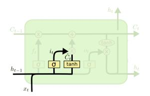
Figure 2.8: The input gate and input activation function. Graphic from [38].
