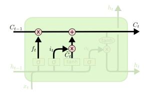
Figure 2.9: The internal cell state of a LSTM. Graphic from [38].
