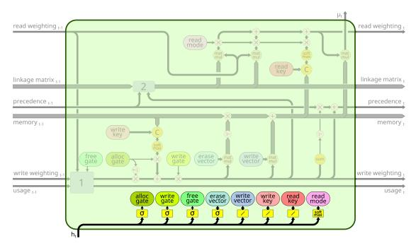
Figure 2.16: The control signals used in the memory unit of a DNC.
