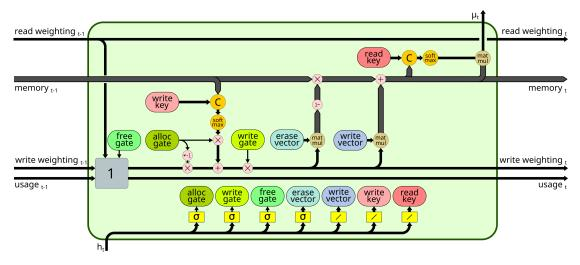
Figure 6.4: The schematic of an content-based memory unit.
