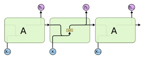
Figure 2.4: A RNN node with a tanh activation function. Black lines show the signal flow.  $h_t$  and  $x_t$  are the output and input signal in each time step t. Graphic from [38].
