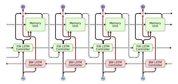
Figure 6.2: The bidirectional controller architecture in the BiDNC setup.
