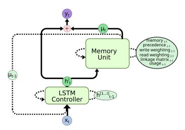
Figure 2.14: The Differential Neural Computer (DNC) with the signal transitions. The dotted lines illustrate recurrent connections.
