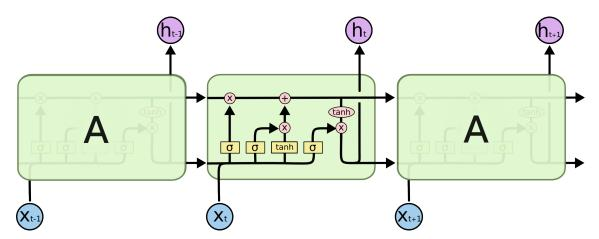
Figure 2.6: The inner function of a LSTM node. Circles with  $\boldsymbol{x}$  and + are signal multiplication and aggregation.  $\sigma$  and tanh are activation functions. Black lines show the signal flow.  $\boldsymbol{h}_t$  and  $\boldsymbol{x}_t$  are the output and input signal in each time step t. Graphic from [38].
