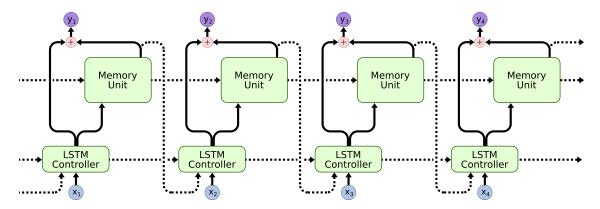
Figure 2.23: An overview of the DNC parts and its signals in unfolded view. The dotted lines illustrate recurrent connections.
