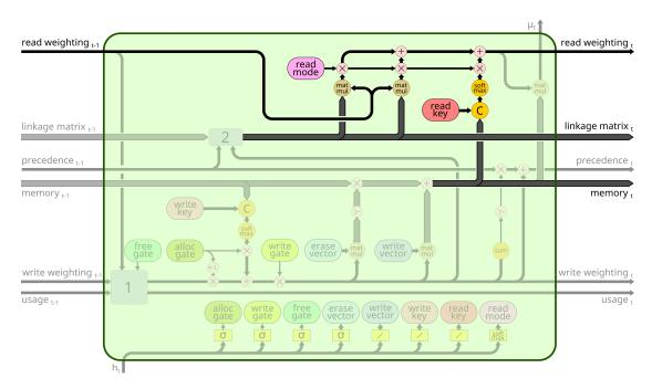
Figure 2.21: The read head, the mechanism to compute the read weightings, the location in the memory from where to read information.
