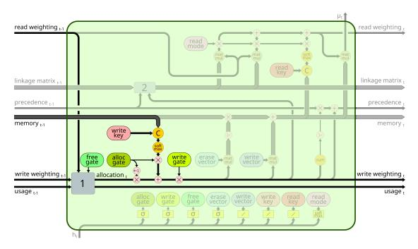
Figure 2.17: The figure shows the mechanism to compute the write weightings. It describes the location in the memory matrix where to add or erase information. The write weightings are computed based on the content-based addressing (write key and the previous memory matrix) and the dynamic memory allocation (the previous usage, read and write weightings and the free gate)
