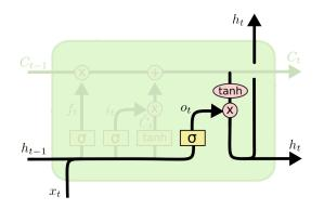
Figure 2.10: The output gate and the activation of the output stream of a LSTM. Graphic from [38].
