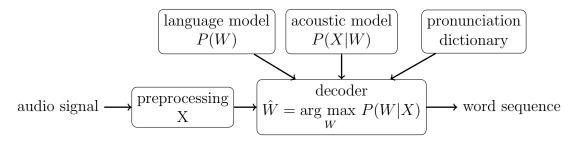
Figure 2.4: Diagram of a speech recognition system
