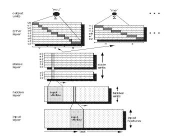
Figure 1. MS-TDNN architecture as used for handwriting recognition.
