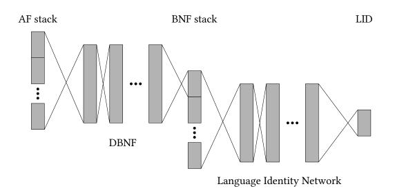
Figure 4.1.: Overview of the network architecture used to extract the Language Identity (LID). The acoustic features (AF) are being pre-processed in a DBNF in order to extract BNFs. These BNFs are being stacked and fed into the second network to extract the LID.
