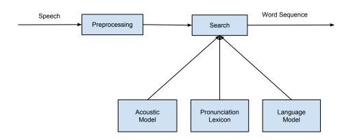
Figure 5.1: Diagram of a HMM based speech recognition system
