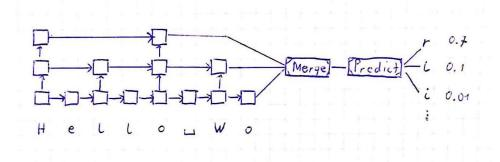
Figure 4.1: Visualization of an unrolled Hierarchical Clockwork RNN
