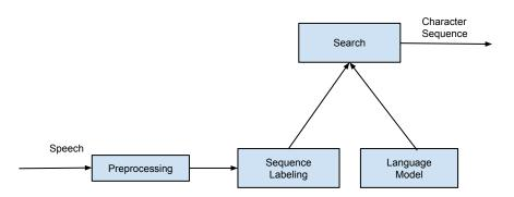
Figure 5.4: Diagram of a CTC based speech recognition system with a language model
