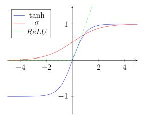
Figure 2.1: Visualization of different activation functions: hyperbolic tangens tanh, sigmoid  $\sigma$  and Rectified Linear Unit ReLU
