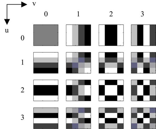
Figure 1. DCT basis functions for  $N = 4$
