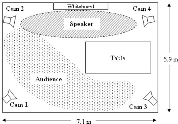
**Figure 1. The smart-room is equipped with 4 fixed cameras at a height of approximately 2.7m. The cameras' joint field-of-view covers the entire room**
