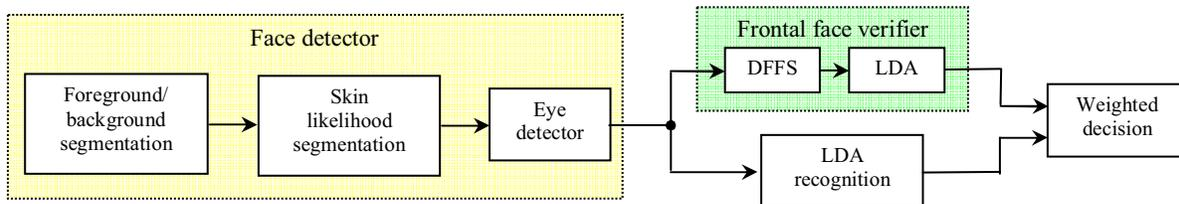
**Figure 6. Block diagram of the AIT end-to-end face recognition system**
