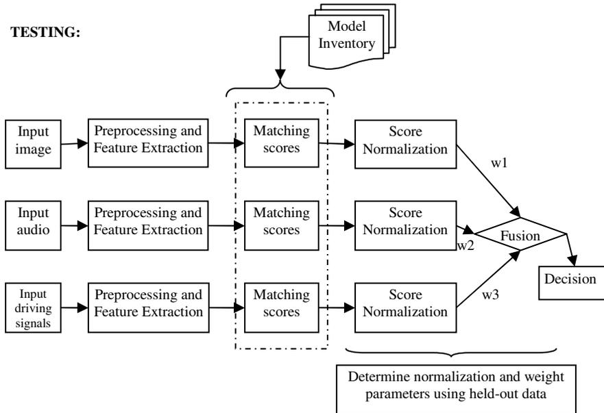
**Fig. 2.** System block diagram for testing the multimodal person recognition system
