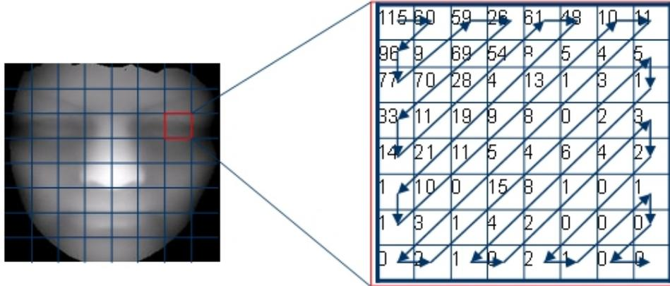
Figure 3.8: Local DCT feature vector from depth image.
