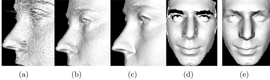
Figure 3.1: (a) Original range image containing spikes and Gaussian noise. (b) Spikes are removed with a median filter. (c) Range image is smoothed with a Gaussian filter. (d) Holes on wet and hairy surface. (e) Hole-filling with linear interpolation.
