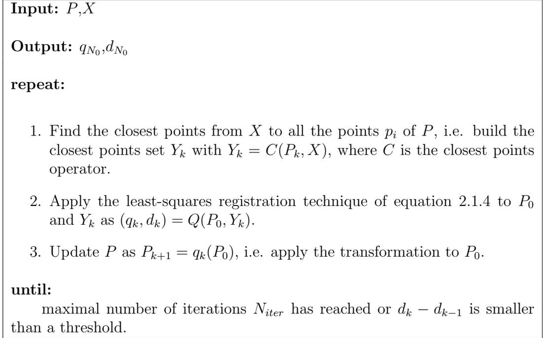
Figure 2.1: The ICP-Algorithm.
