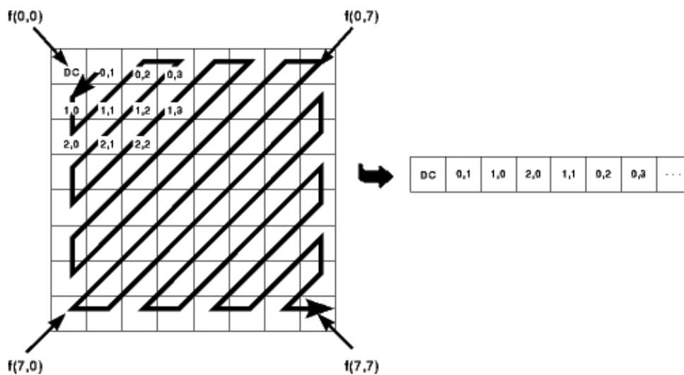
Figure 2.7: Zig-zag scanning, first coefficient is average intensity value of this block (DC).
