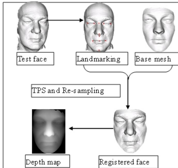
Figure 3.6: Face registration and depth map image generation.
