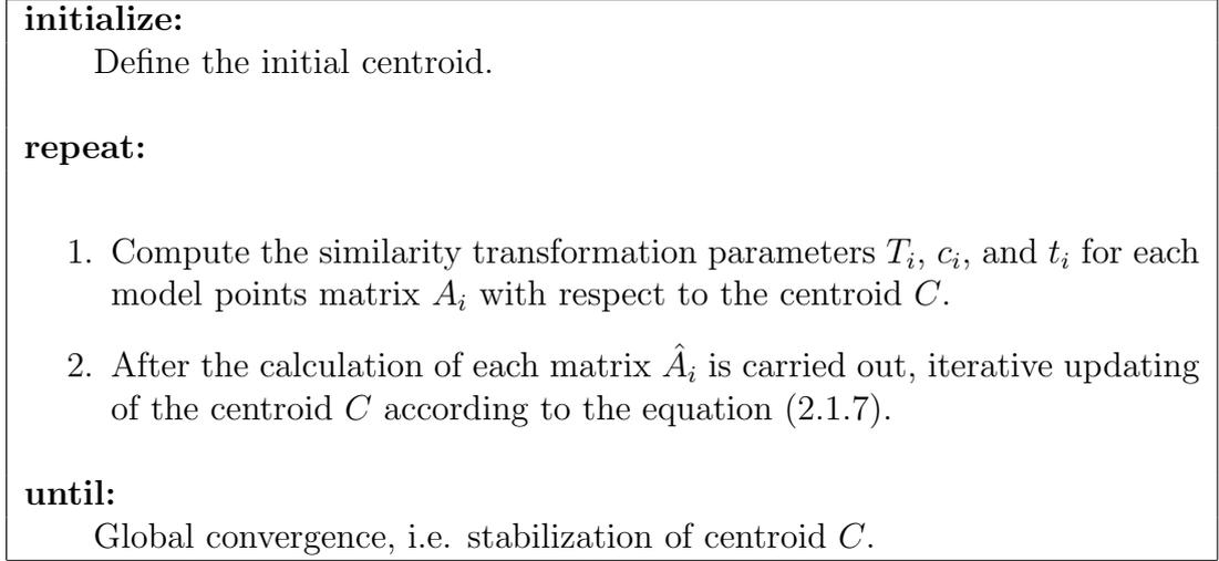
Figure 2.3: Algorithm for the Generalized Procrustes analysis
