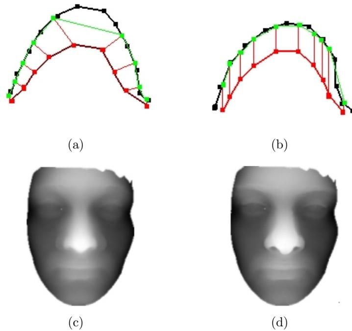
Figure 3.5: (a) Closest-point mapping, find the closest point on target mesh for each base mesh vertex. (b) Ray-casting mapping, find the crossing point on target mesh for each ray casting from base mesh vertices. (c) Depth map constructed with closest-point mapping. (d) Depth map constructed with ray-casting mapping.
