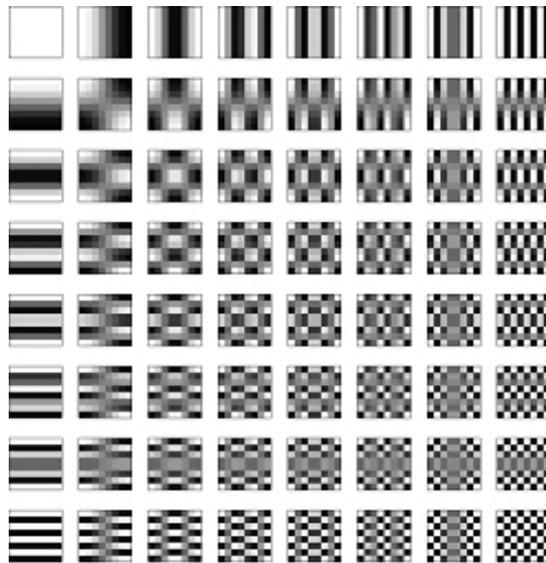
Figure 2.6: DCT basis functions for  $N = 8$ , The origin is at the top left corner.
