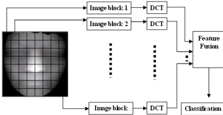
Figure 3.9: Local feature combination at the feature level.
