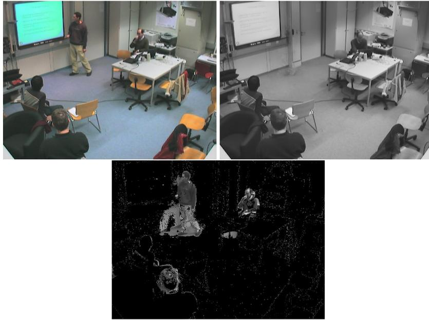
Figure 3.4: On the top left is the original camera image, on its right side the adapted background image that is updated every second and on the bottom the resulting foreground image (black being the background).
