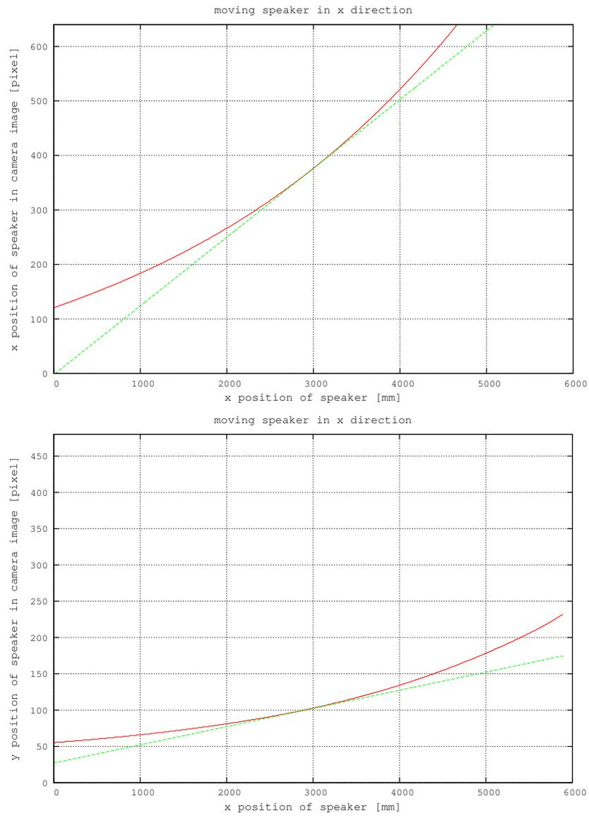
Figure 3.2: Comparison between nonlinear function and first order Taylor series. On the top the global  $x$  position of the speaker is plotted against the  $x$  position in the camera image. On the bottom it is plotted against the  $y$  position in the camera image.
