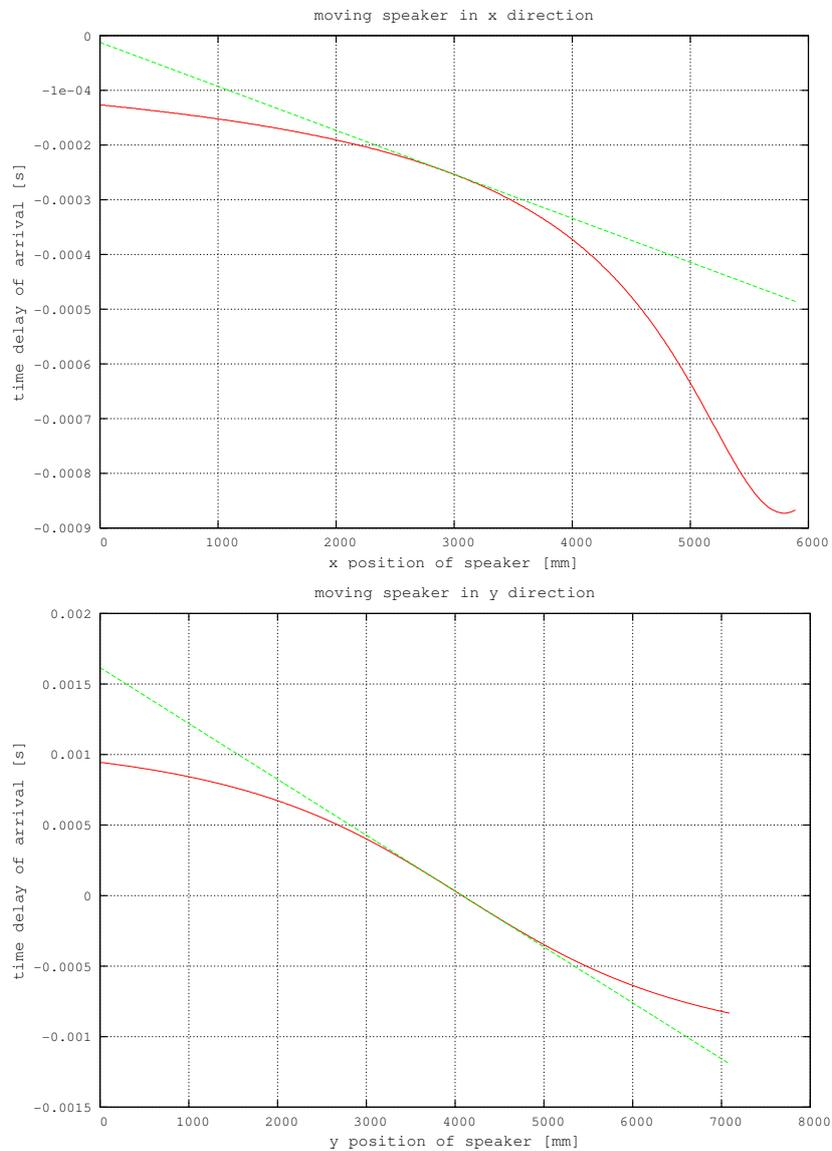
Figure 2.2: Comparison between nonlinear function and first order Taylor series. On the top the microphones used are on top of each other and the speaker is moving in the  $x$  direction. On the bottom the microphones are beside each other and the speaker is moving in the  $y$  direction.
