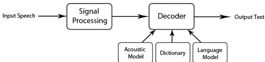
Figure 1.1: Block diagram of a standard ASR system.
