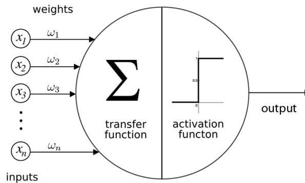
Figure 3.2: Processing pattern within a neuron.
