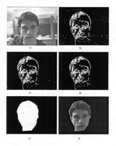
Figure 3.6: *Background subtraction*. a) the original image, b) motion over a few frames, c) applied noise filter to motion image, d) detected head outline, e) solid head mask, f) the original head image with a blue screen background
