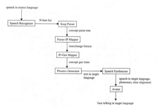
Figure 4.2: The Janus III machine translation system plus the avatar for audio-visual output.
