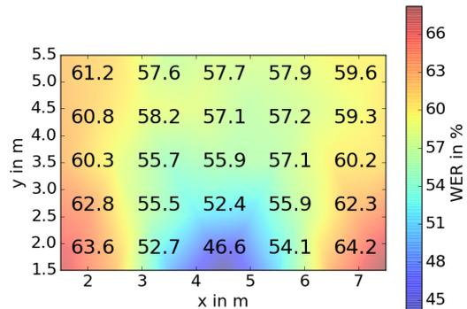
**Figure 2:** WER depending on receiver position for a system trained with the RIRs from the room. The source was positioned at (4,5 m, 0,5 m) and the total size of the room is  $7.5 \text{ m}^3 \times 9 \text{ m}^3 \times 3.5 \text{ m}^3$ .
