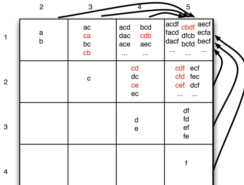
Figure 4.4.: Schematic overview of cyk with marked partial hypothesis immune from pruning
