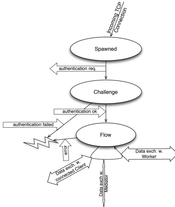
Figure 3.5.: State graph of client processes
