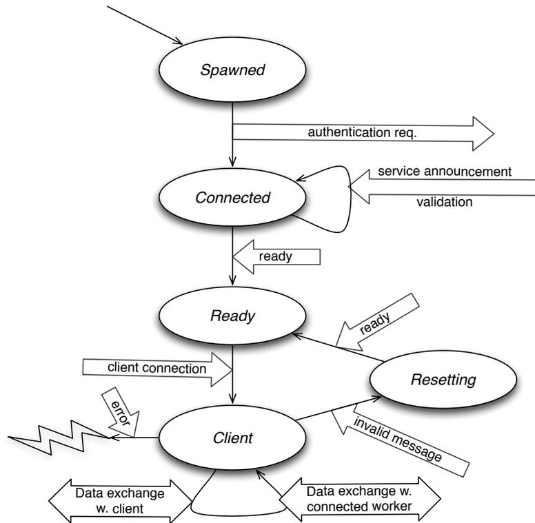
Figure 3.4.: State graph of worker processes
