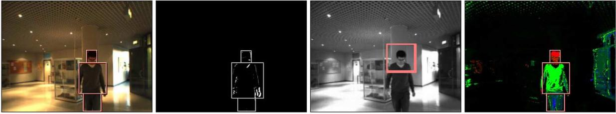
Fig. 3. Video feature maps with the 3-box body model superimposed. (a) Camera image, (b) Foreground segmentation. (c) Detector response. (d) Color segmentation (head–torso–leg color model projected to the red–green–blue channel, respectively).
