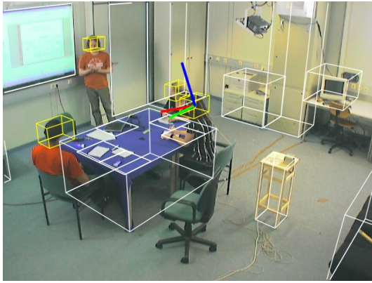
Figure 4: Camera 1’s view of a recorded meeting scene during a short presentation, given by person P00. Person P02, sitting opposite to the presenter, is wearing the magnetic motion sensor to capture her true head orientation, depicted by the red (x), green (y) and blue (z) coordinate axes. All axis aligned bounding boxes of focus targets we annotated, visible from this view, are highlighted in white.
