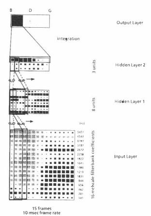
Fig. 2. The architecture of the TDNN.
