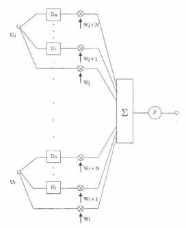
Fig. 1. A Time-Delay Neural Network (TDNN) unit.
