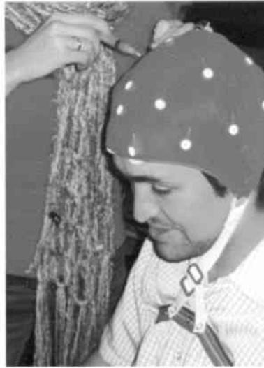
Figure 2.7: Electro-Cap being filled with a conductive gel
