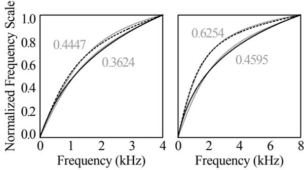
**Fig. 1.** The approximations of Mel-frequency (black lines) and Bark-frequency (dotted black lines) by the bilinear transformation (gray lines including the warping factor in gray digits) are demonstrated for 8 and 16 kHz sampling rates.
