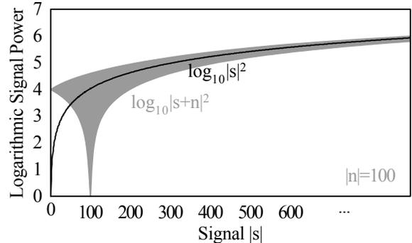
**Fig. 3.** Comparison of the power to the logarithmic power of the clean signal  $s$ , black line, and the influence of additive noise  $n$ , gray area.
