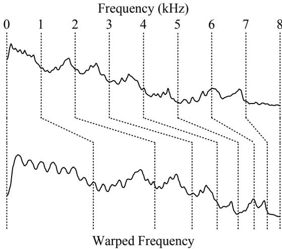
**Fig. 2.** Comparison of MVDR (top) and Mel-warped-MVDR (bottom) spectral envelopes, both of same model order 120.
