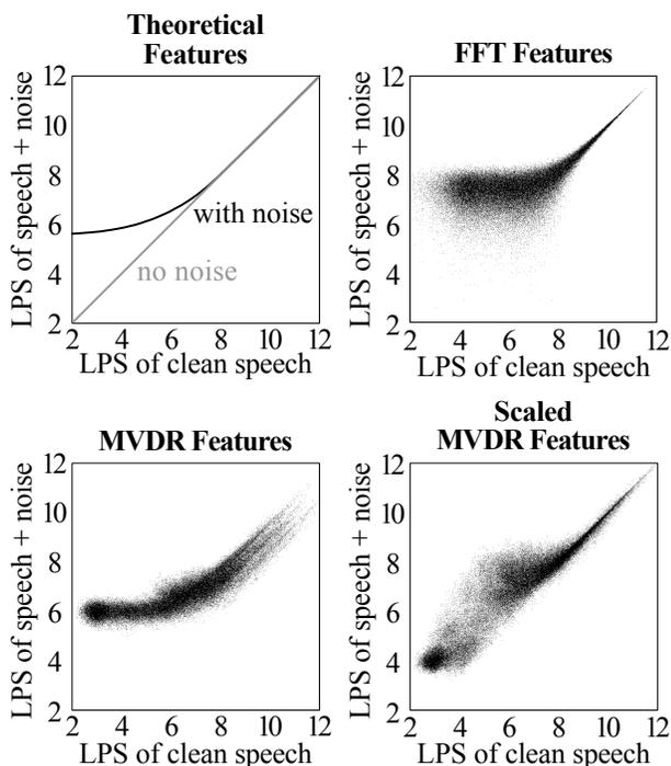
**Fig. 4.** Shown are the influence of noise (signal to noise ratio = 8dB) in the *logarithmic power spectrum* (LPS) on the features for different spectral estimation methods in dependence of their signal energies.
