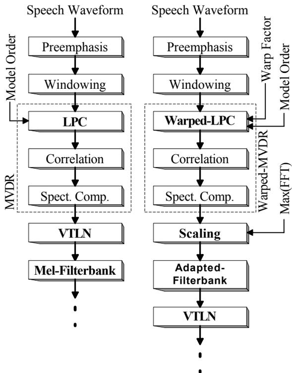
Fig. 6. Extract of the MVDR (left) and the warped&scaled-MVDR (right) acoustic preprocessing as used in our experiments.
