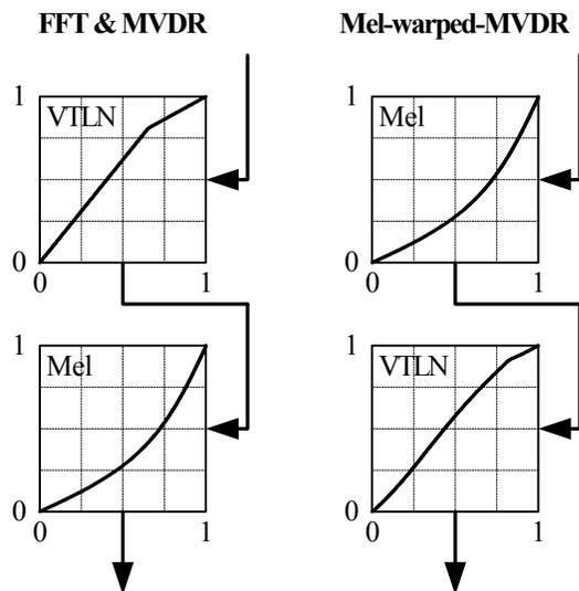
**Fig. 7.** Shown are the linear and the Mel-warped-VTLN approaches. Note that the VTLN has to be implemented in different manners.
