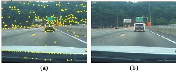
**Figure 9. False positive examples of road sign localization.**
