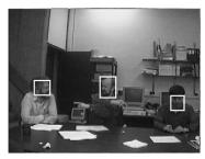
Figure 6 Locating faces using a combination of color, geometry, and motion information
