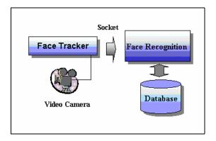
Figure 4. Architecture of the face recognition system
