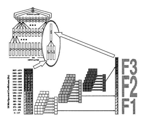
Figure 1: The Frequency Shifting TDNN (FSTDNN) architecture.
