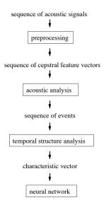
Figure 1: System structure for explicit time modeling with neural networks
