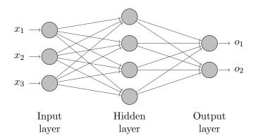
Figure 2.2.: Architecture of a multi-layer perceptron with a single hidden layer.
