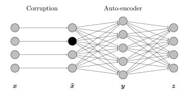
Figure 2.5.: Architecture of a denoising auto-encoder with masking noise. The black color indicates that units are set to zero (masked).
