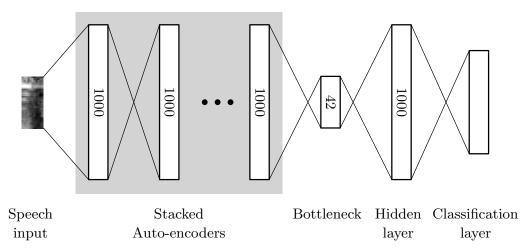
Figure 3.1.: The proposed architecture contains a number of equally-sized layers pretrained as denoising auto-encoders. The bottleneck, an additional large hidden layer and the classification layer are added prior to supervised fine-tuning.
