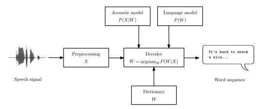
Figure 2.1.: Basic components of a speech recognition system
