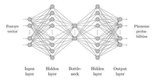
Figure 2.3.: Multi-layer perceptron for bottleneck feature extraction as proposed by Grézl et al.
