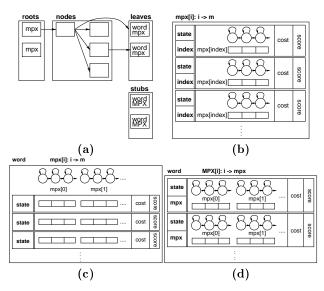
Figure 1. (a) Prefix search tree consisting of roots, nodes, leaves and single phone word nodes [stubs]. The heap structure of a root node (b), a leaf node (c), and a stub (d): state=finite state machine grammar state; mpx=multiplexer; MPX=multiplexer of multiplexers; cost=FSM lookahead score; score=total best score of hypothesis (acoustic plus expected FSM cost).
