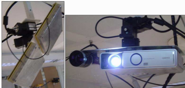
Figure 4. Targeted audio device (left) and a camera-projector pair (right) mounted on motorized computer-controlled pan-tilt units are used as interaction devices in the smart meeting room.
