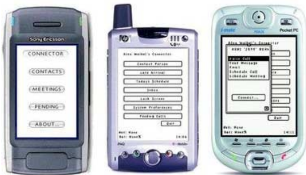
Figure 3. Three generations of smart CHIL phones running the Connector graphical interface: Sony Ericsson P900, HP iPAQ h6315 and i-mate PDA2K GSM/GPRS Pocket PC.
