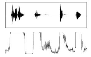
Figure 1: audio signal and output of speech detector
