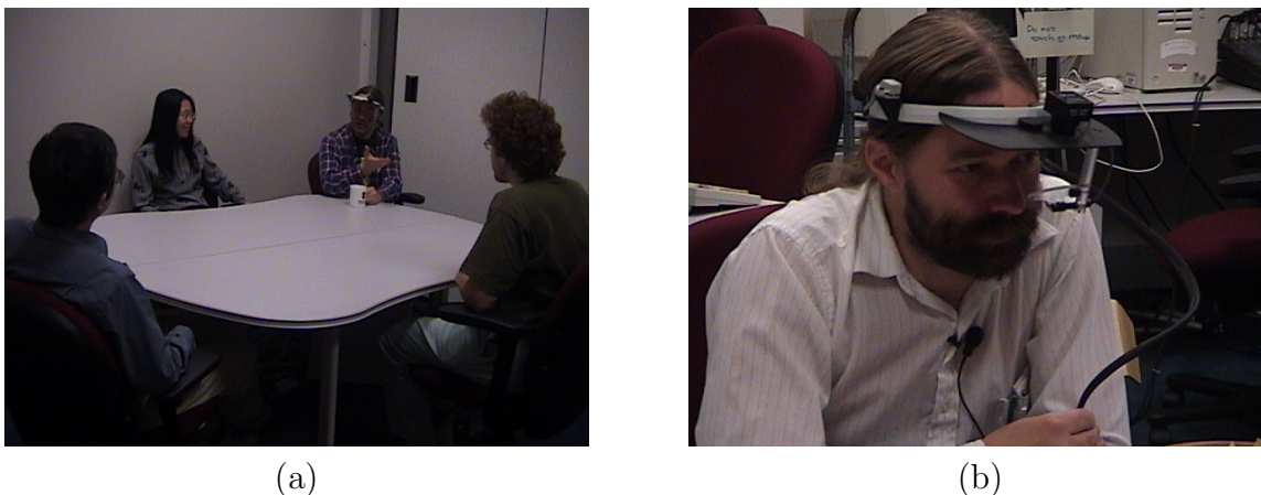
Figure 6.1: a) Datacollection with eye and head tracking system during a meeting. b) A participant wearing the head-mounted eye and head tracking system.
