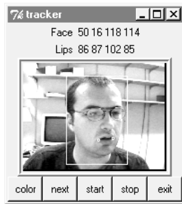
Figure 5 Facial Feature Tracking Application for extracting lips-regions written with the API in TCL/TK
