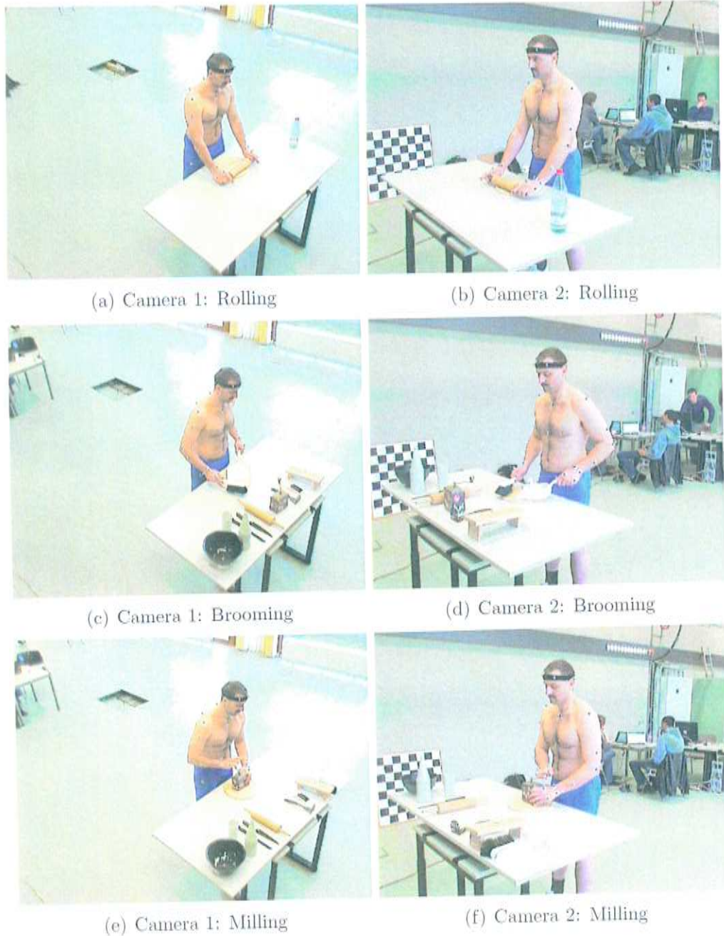
Figure 4.14: Tracking sequences. For the tracking and classification experiments the database from [HK08] was used. It contains several types of motion, captured with a VICON motion capturing system and four Sony VWF 500 color cameras (resolution 640x480). In this figure snapshots of 3 motions (rolling, brooming and milling) are depicted from 2 views each.
