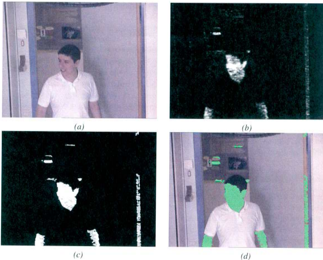
Figure 3.3: Skin segmentation process (a) input image (b) backprojection (c) thresholded back-projection (d) result
