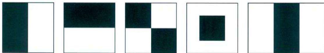
Figure 2.1: Examples of Haar-like features. Their values represent the intensity differences between the black and the white areas.
