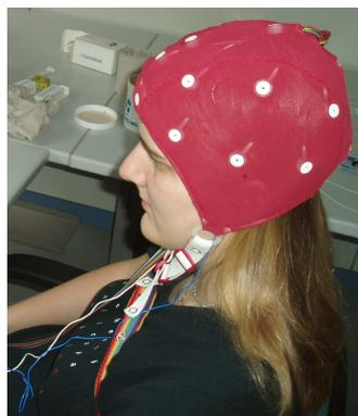
Figure 5.1: The ElectroCap<sup>TM</sup> EEG-cap used for the data collection conducted for this work.
