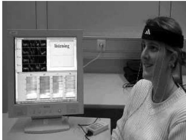
Figure 6.8: The prototype system for user state identification. In the upper left corner of the monitor the recorded EEG signals are displayed, the hypothesis for the current user state can be seen in the upper right corner. The spectrograms for the electrodes Fp1, Fp2 F7 and F8 are shown at the bottom.
