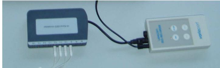
Figure 5.3: The Varioport™ EEG amplifier. Left: the actual amplifier, right: the recorder which controls the amplifier, stores recorded data and established the connection to a computer.
