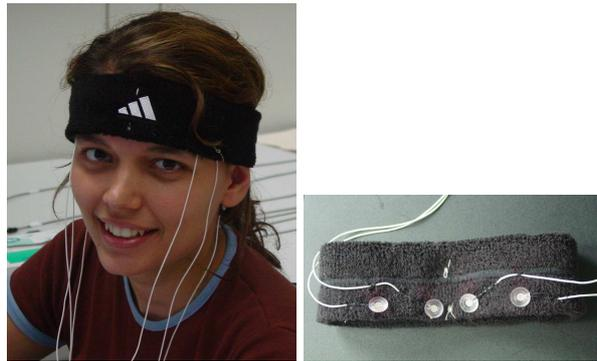
Figure 5.2: Headband for EEG recording (left), electrodes attached on the headband at positions Fp1, Fp2, F7 and F8 (right).
