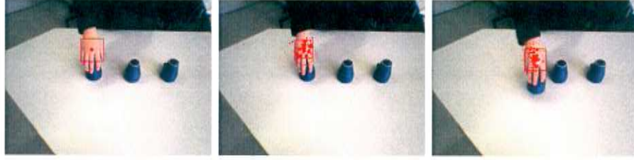
Figure 7: The fleeing-particles problem solved. Frames 0, 21, and 46 show how the particles stayed at the correct depth instead of moving away from the camera. The red dots represent single hypotheses, the red rectangle the perspective projection of the joint hypothesis. The sequence was captured with 30 frames per second.
