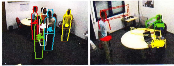
Fig. 2. Audio-visual tracking of multiple persons. Targets are described by an appearance model comprising shape and color information, and tracked in 3D using probabilistic representations [4]. The system tracks 5 people in real-time through multiple persistent occlusions in cluttered environments.
