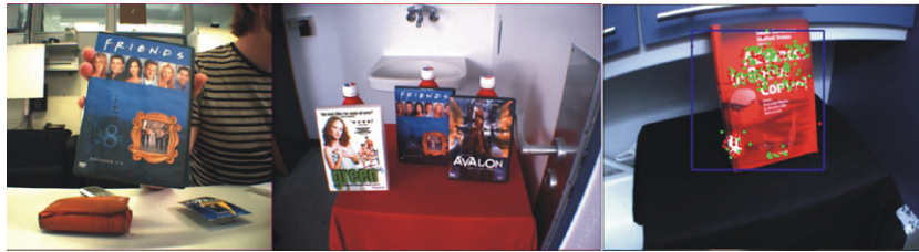
Fig. 4. Snapshots taken from the robot camera. From left to right: object held in front of the robot's camera, multiple objects recognition, unknown object recognition during the experiment with feature extraction and shape segmentation.
